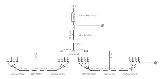
The maximum allowable distance between points A and B for expansion is 15 meters, without considering voltage drop interference in the distribution.
