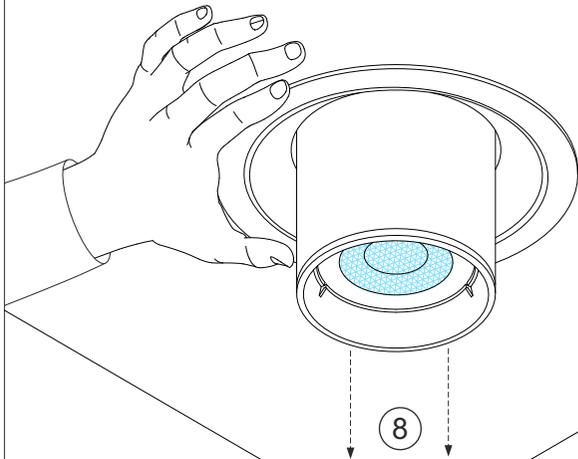
tilting is capable only when the main body is full extracted
