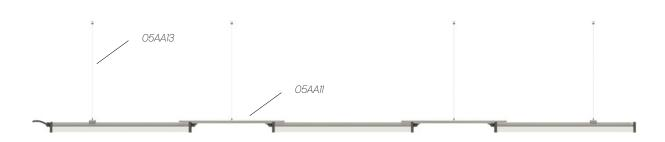
Thanks to the O5AAII accessory you can install the devices in suspended continuous line by avoiding the use of busbars or cable raceways. This bracket serves as the mechanical joining, allows the masking of the connection cable between two devices and reduces the suspension points. It is click fixed on the devices and can be cut at the construction site.
